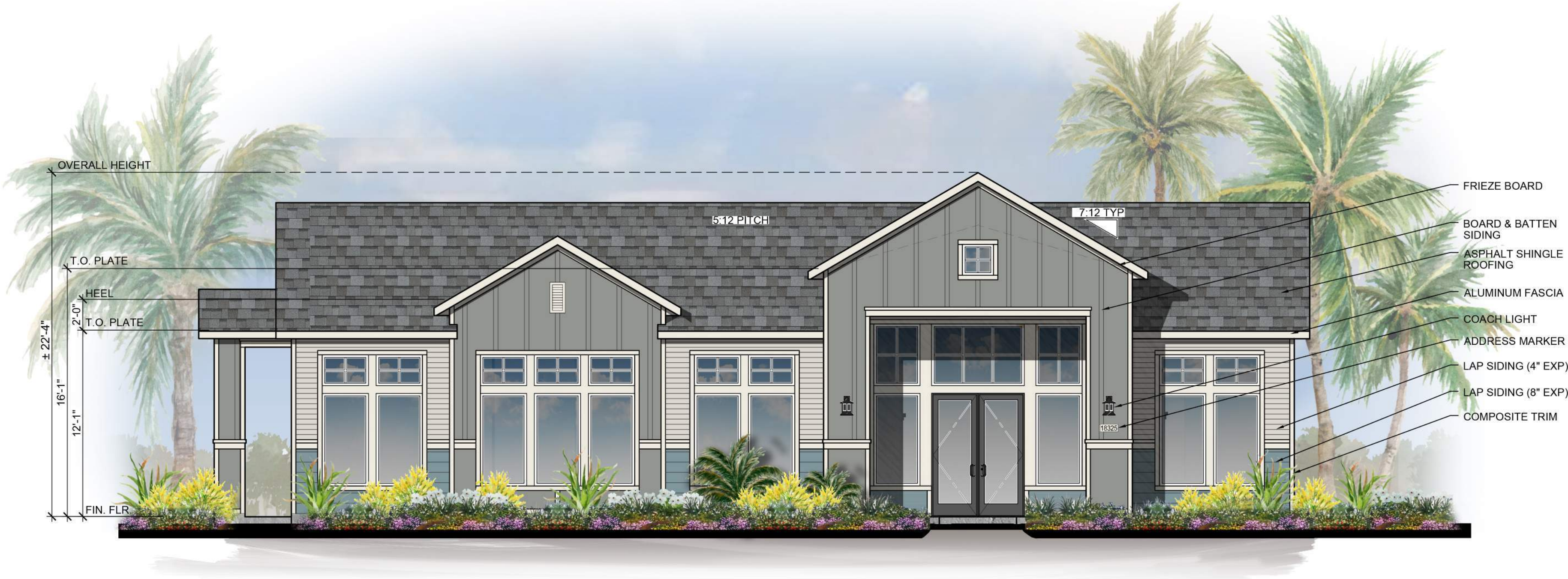
FRONT ELEVATION COASTAL 3/16" = 1'-0"
