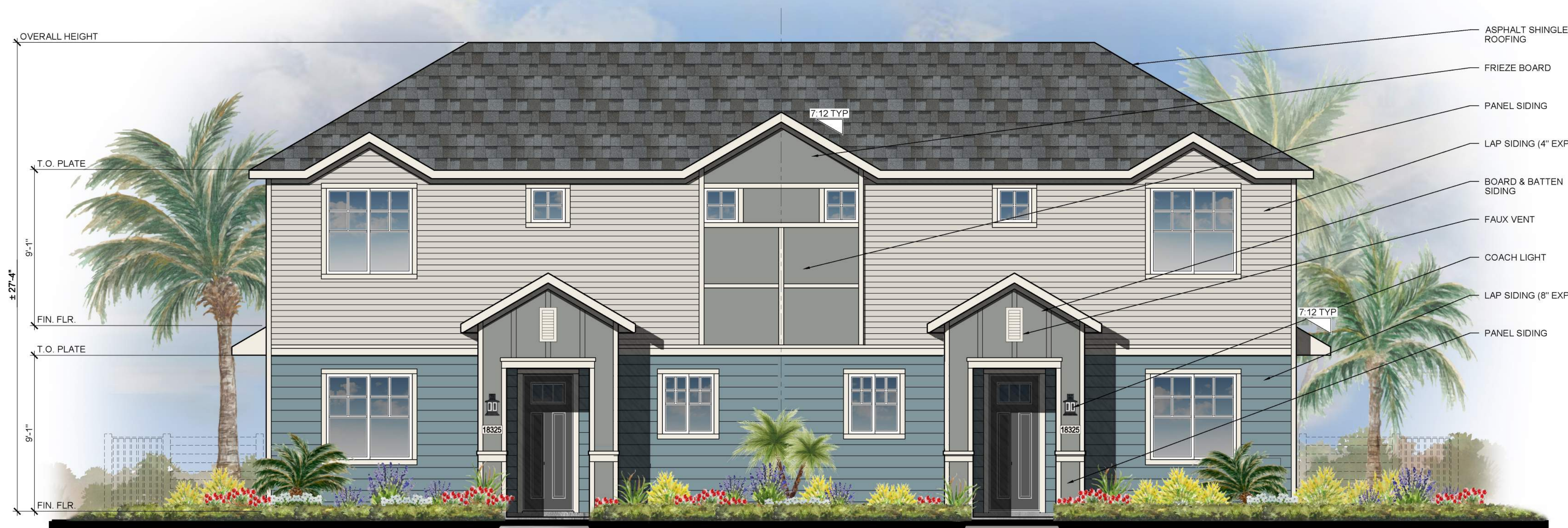
FRONT ELEVATION COASTAL STYLE 1/4" = 1'-0"
