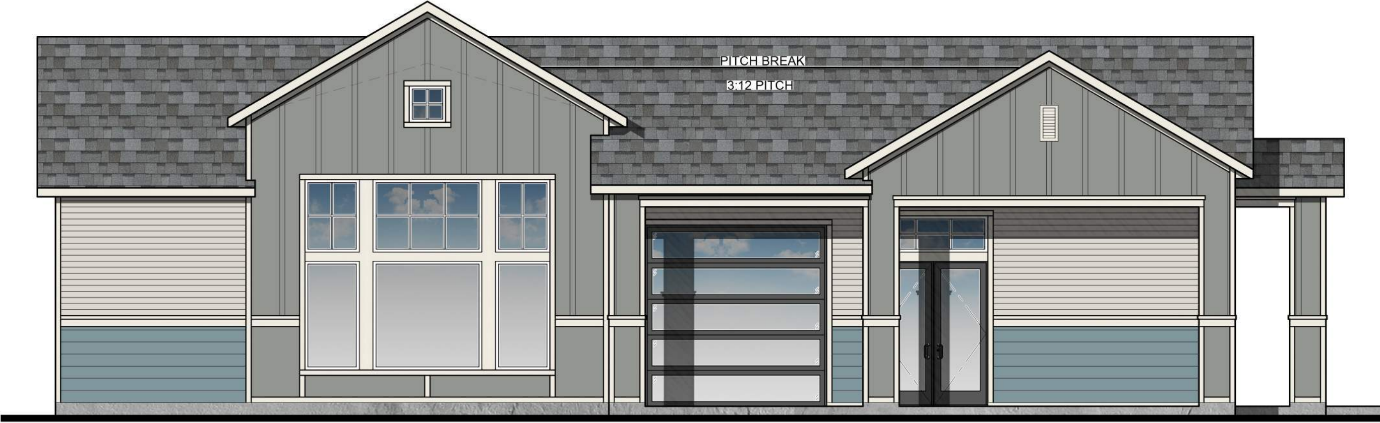
REAR ELEVATION COASTAL 3/16" = 1'-0"
