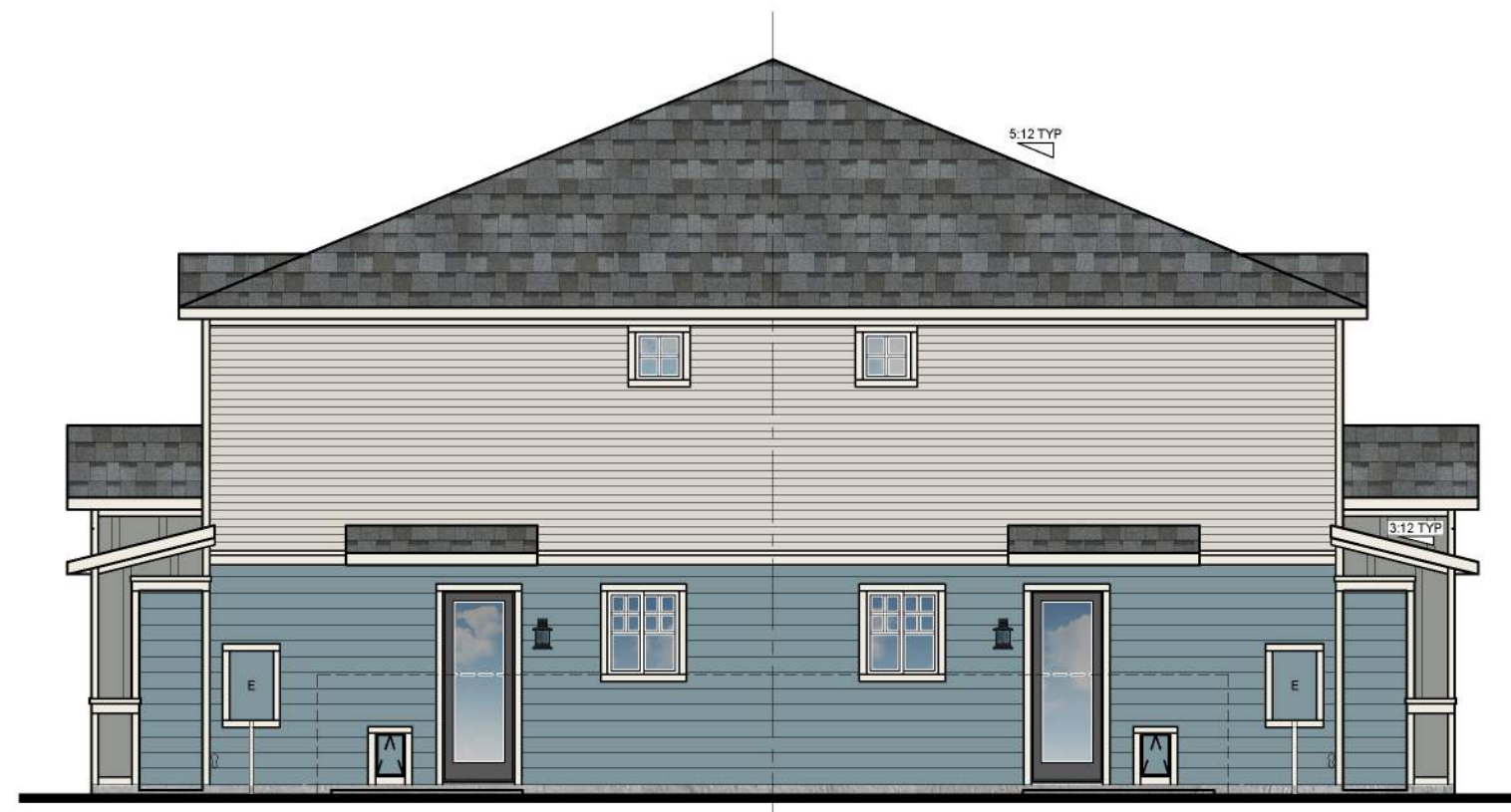
LEFT ELEVATION COASTAL STYLE 1/8" = 1'-0"
