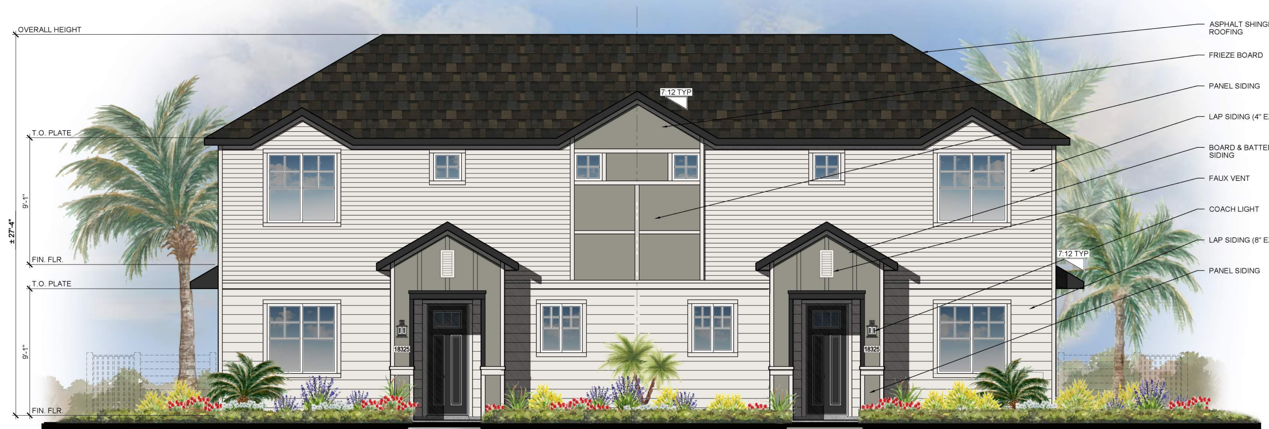
FRONT ELEVATION COASTAL STYLE 1/4" = 1'-0"
