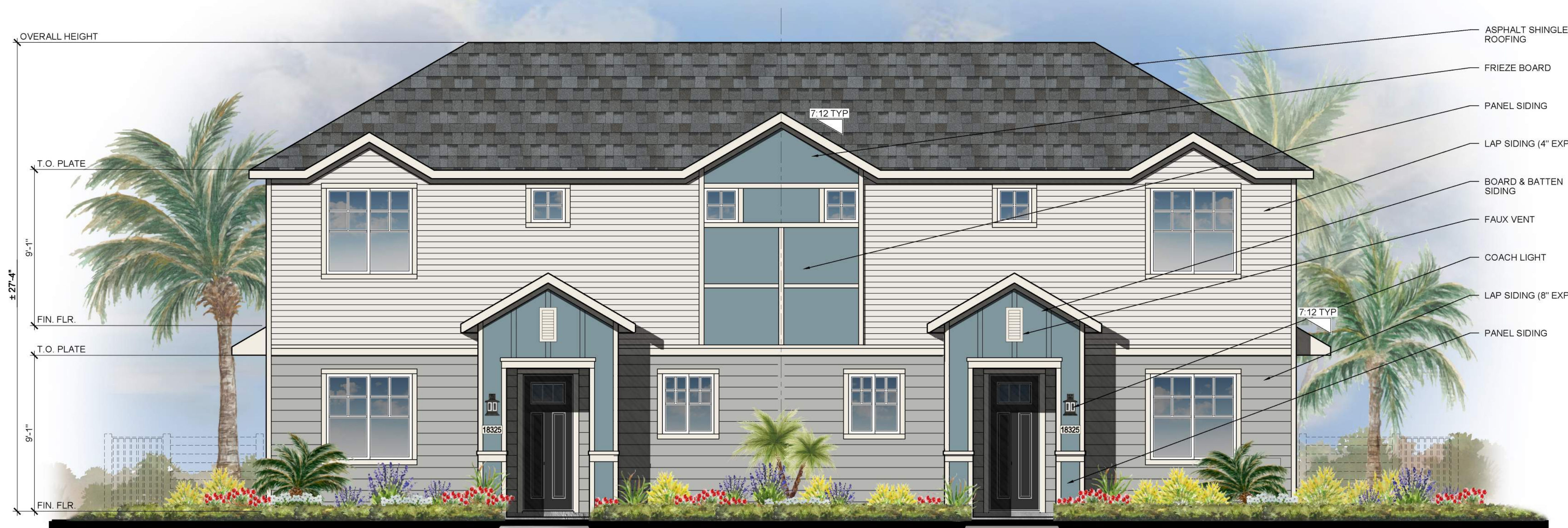
FRONT ELEVATION COASTAL STYLE 1/4" = 1'-0"
