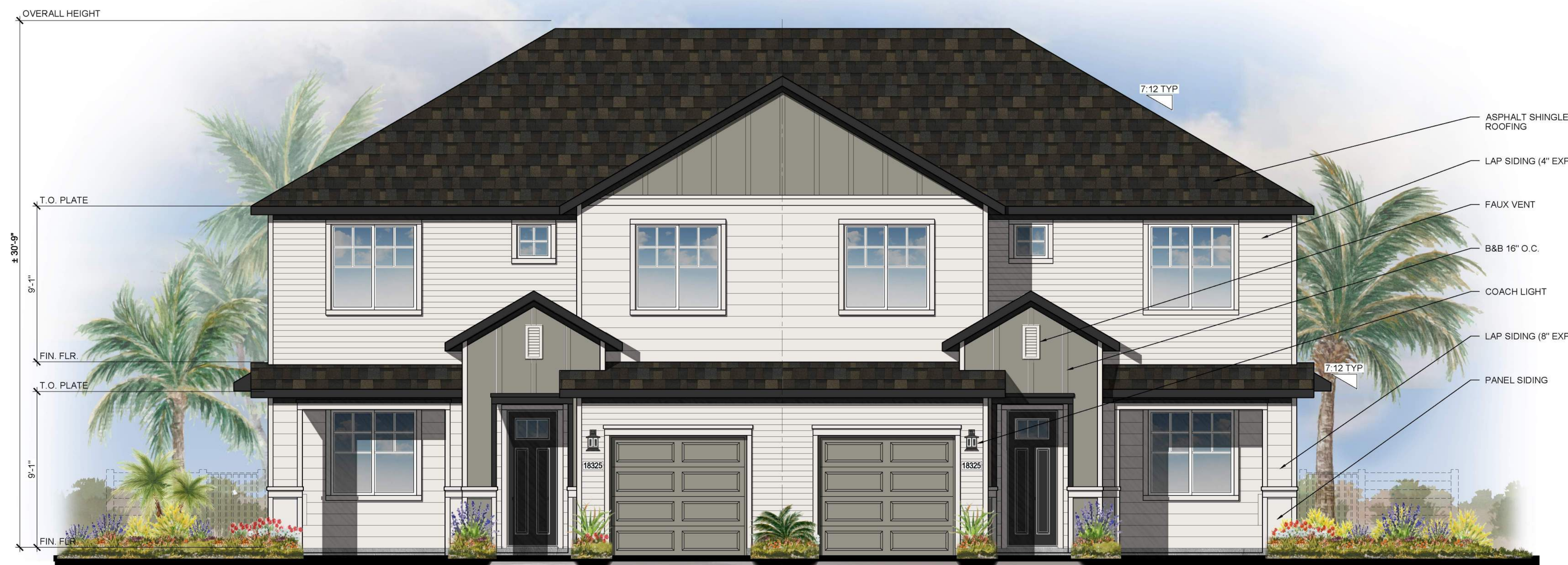
FRONT ELEVATION COASTAL STYLE 1/4" = 1'-0"
