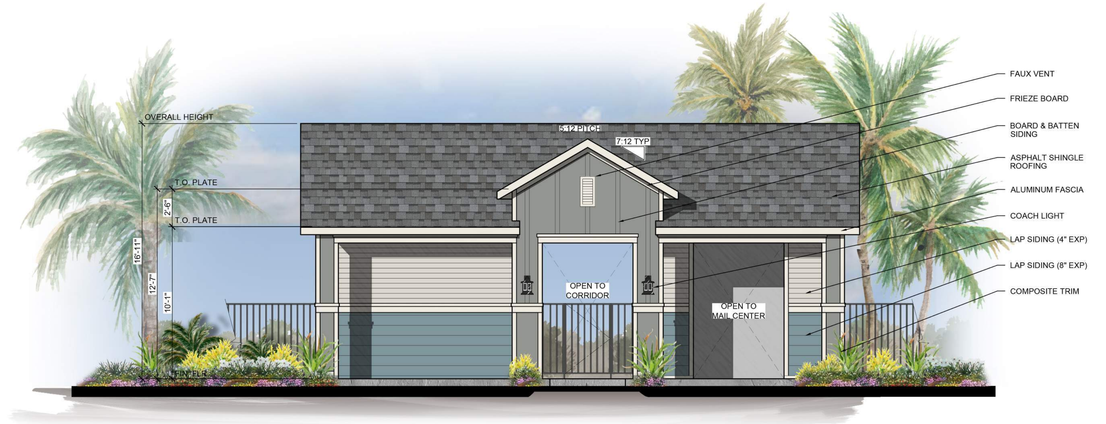
FRONT ELEVATION COASTAL 1/4" = 1'-0"
