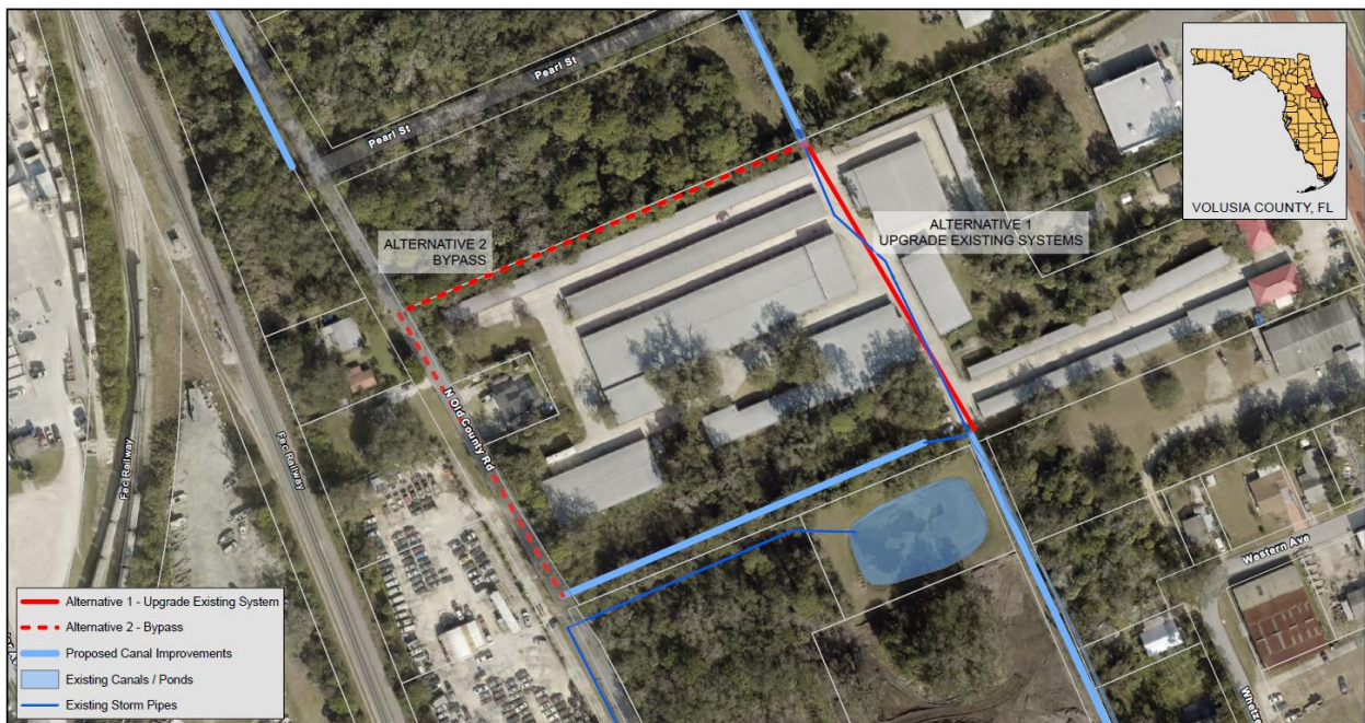
Group A Improvements Figure A2 - EW Storage Upgrade / Bypass
